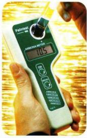
evels of ammonia in industrial effluents can be checked quickly with a handheld photometer developed by **Palintest**. Samples can be taken from any point in the treatment process and tested in a couple of minutes.
