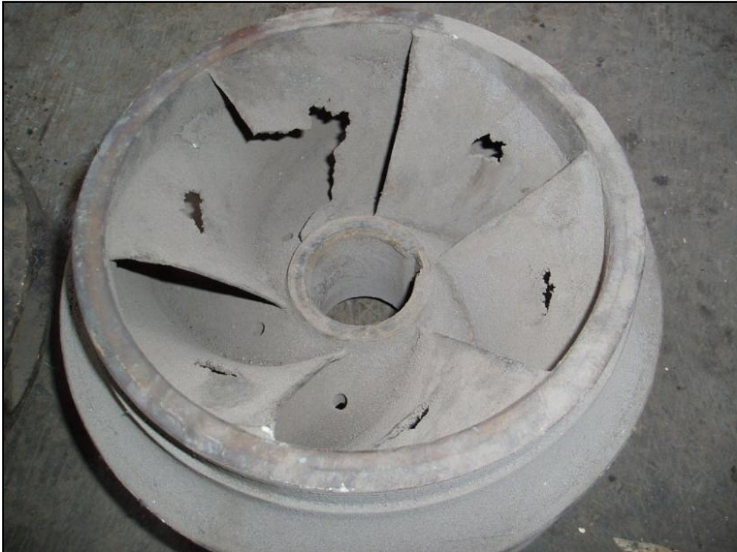
Cavitation damage in an impeller
