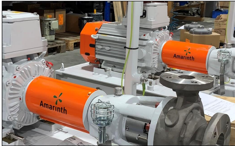
Amarinth API 610 titanium pumps on bespoke baseplates ready for shipment to VWS Westgarth
