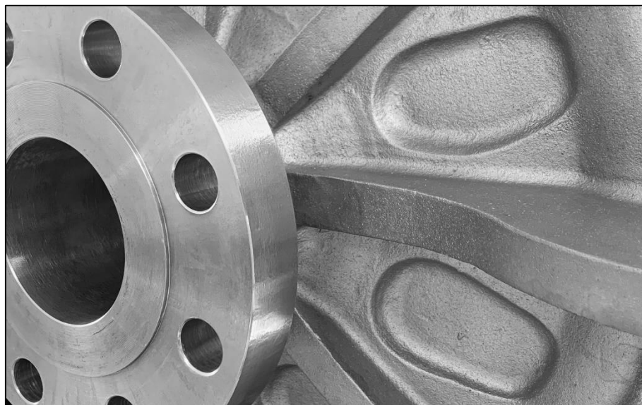
Close-up of titanium casing on Amarith API 610 pump manufactured for VWS Westgarth
