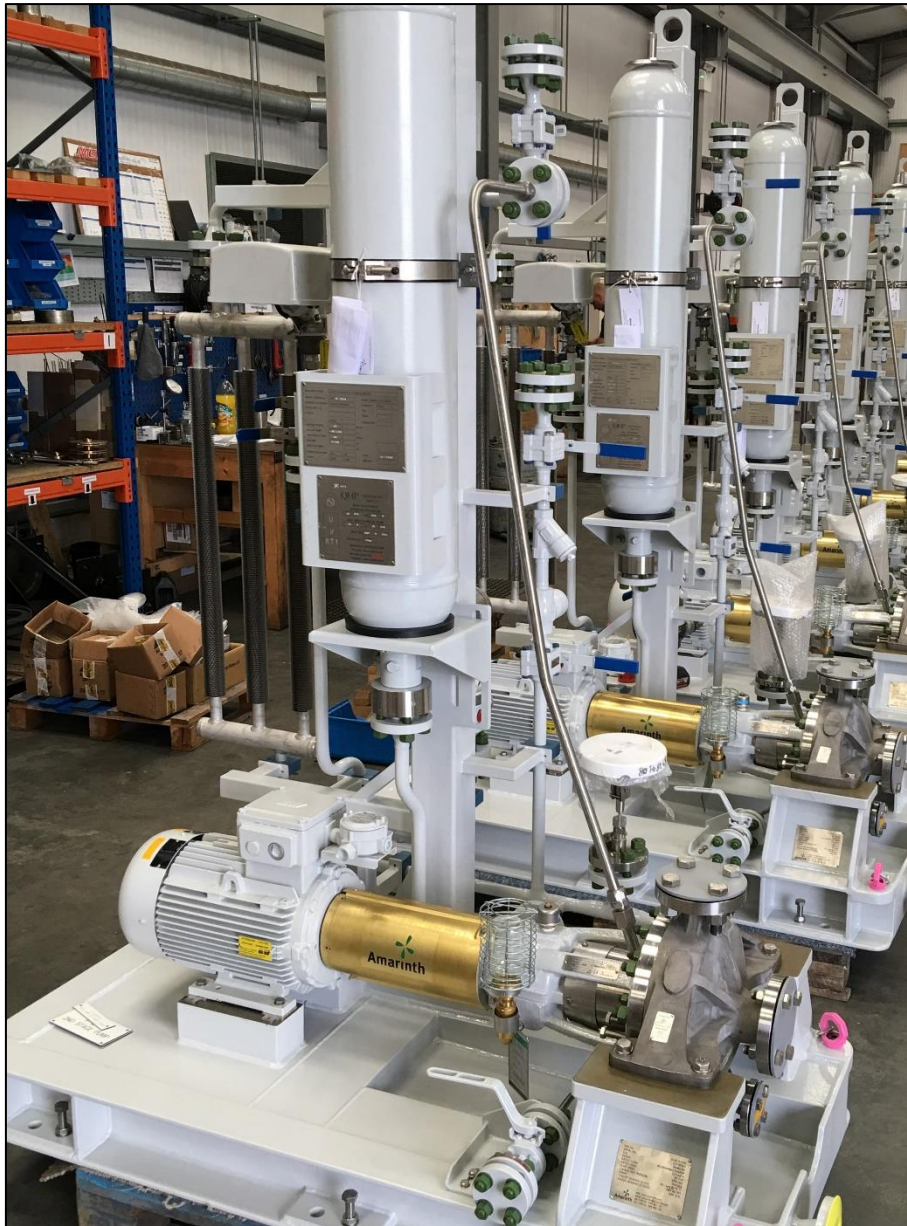
Amarinth API 610 OH2 pumps being assembled for Karachaganak Petroleum Operating
