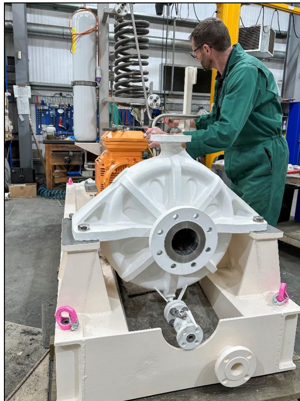
Amarinth API 610 12 th Edition OH2 pumps being readied for final witness and packing before transportation to the North Sea
