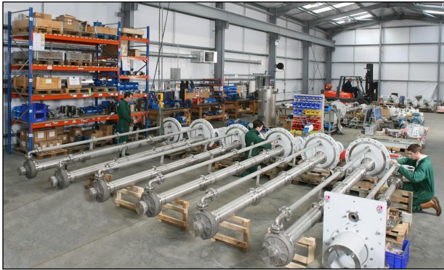
Amarinth engineers undertaking API 610 VS4 pump assembly
