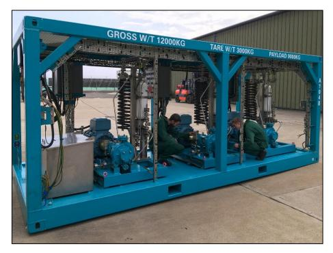
Amarinth engineers start inspecting the first OSRL oil containment skid to arrive with its three Amarinth API 610 OH1 pumps and Plan 53B seal support systems
