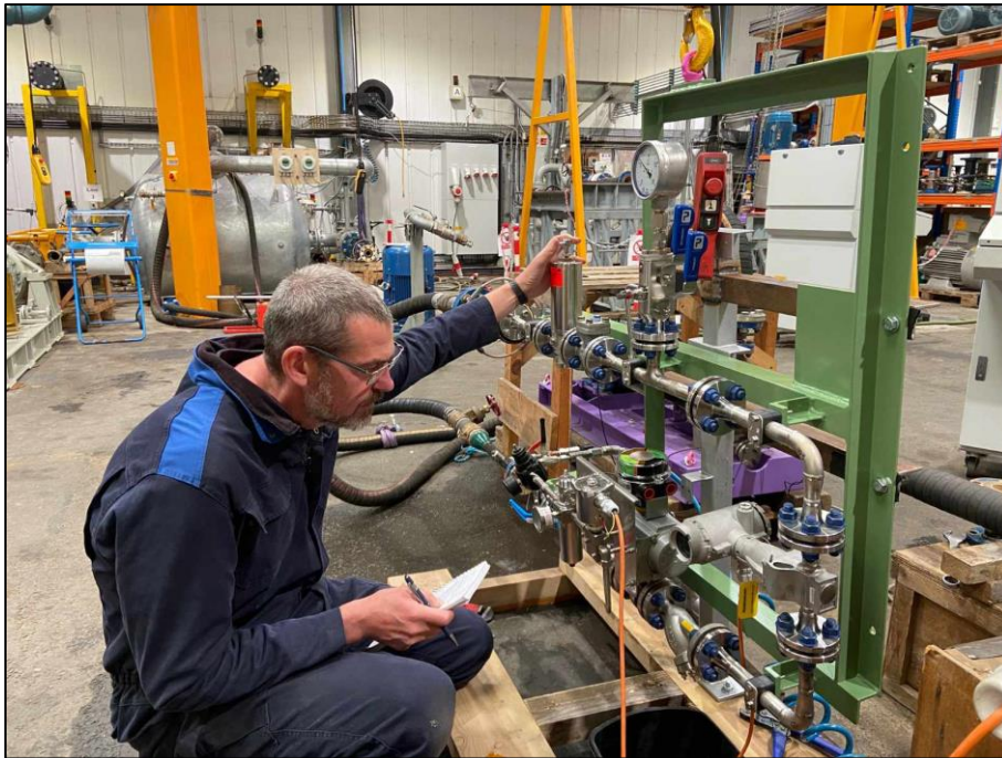
Amarinth engineer testing an external flush panel
