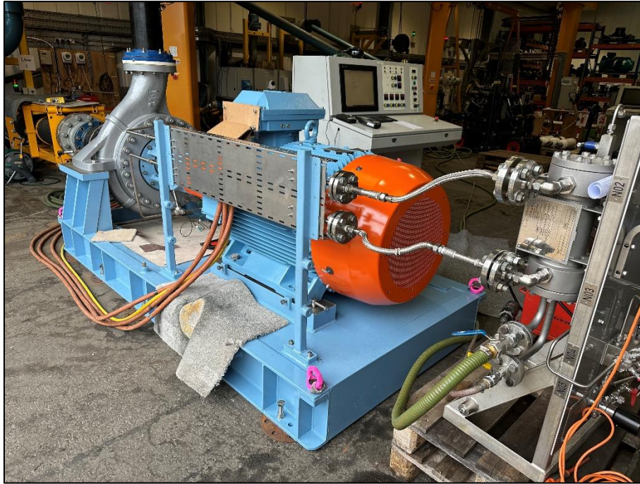
API 610 OH2 pump for FPSO Atlanta undergoing final testing at Amarith's facilities
