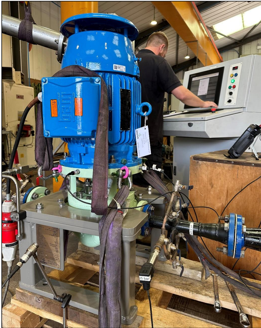
Amarinth API 610 OH5 Vertical In-Line pump for Siemens Energy undergoing hydrodynamic testing
