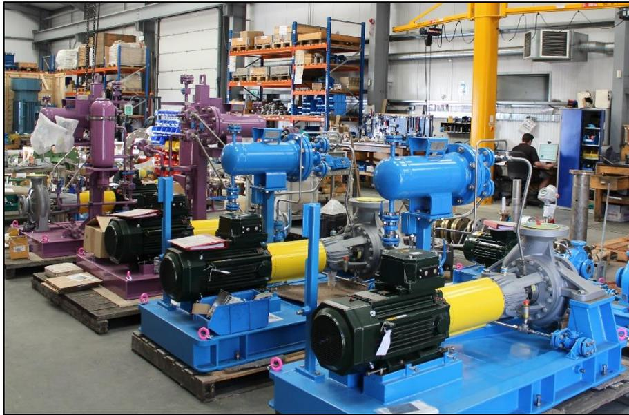
Amarinth API 610 OH2 pumps with bespoke forced air-cooling Plan 53B seal support systems being readied for shipment to the WARA Pressure Maintenance project
