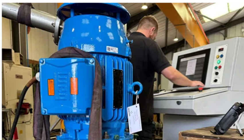
An Amarith API 610 OH5 Vertical In-Line pump for Siemens Energy undergoing hydrodynamic testing
