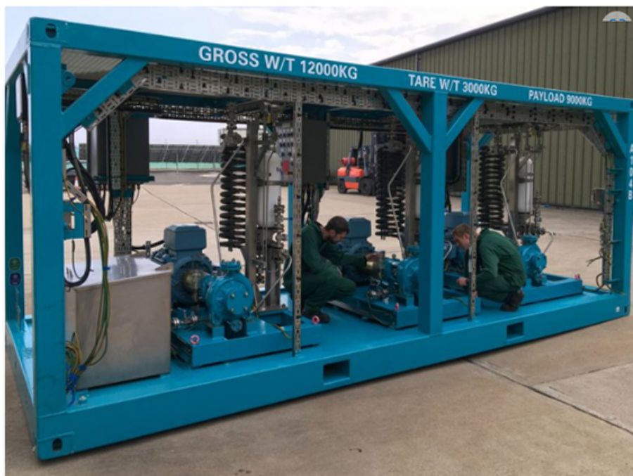
Amarinth engineers start inspecting the first OSRL oil containment skid to arrive with its three Amarith API 610 OH1 pumps and Plan 53B seal support systems. (Image source: Amarith Limited)
