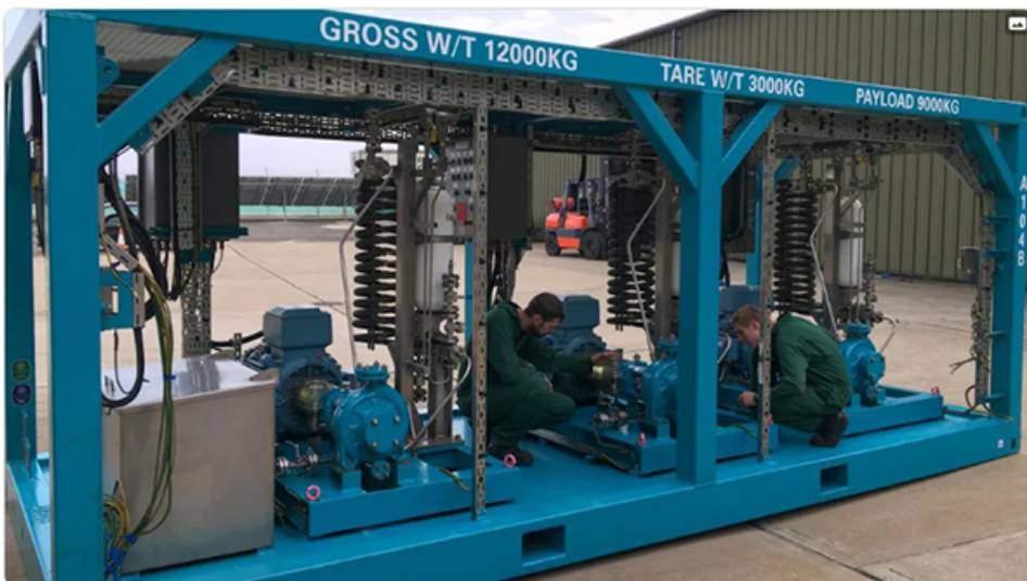
Amarinth engineers start inspecting the first OSRL oil containment skid to arrive with its three Amarith API 610 OH1 pumps and Plan 53B seal support systems.
