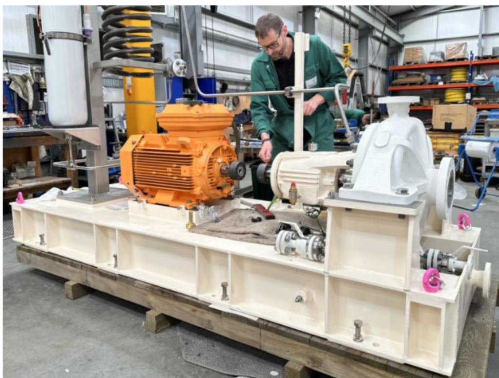
Amarinth API 610 12th Edition OH2 pumps being readied for final witness and packing before transportation to the North Sea (Image source: Amarith Ltd.)
