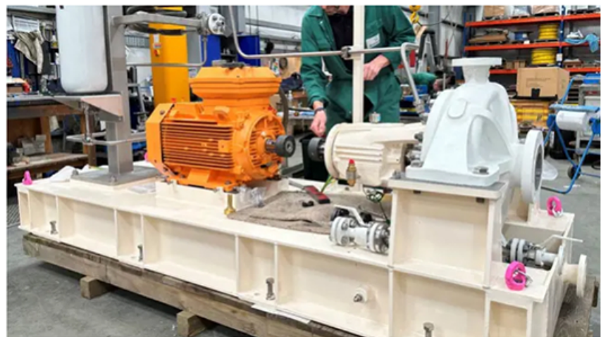
Amarinth API 610 12th Edition OH2 pumps being readied for final witness and packing before transportation to the North Sea.
