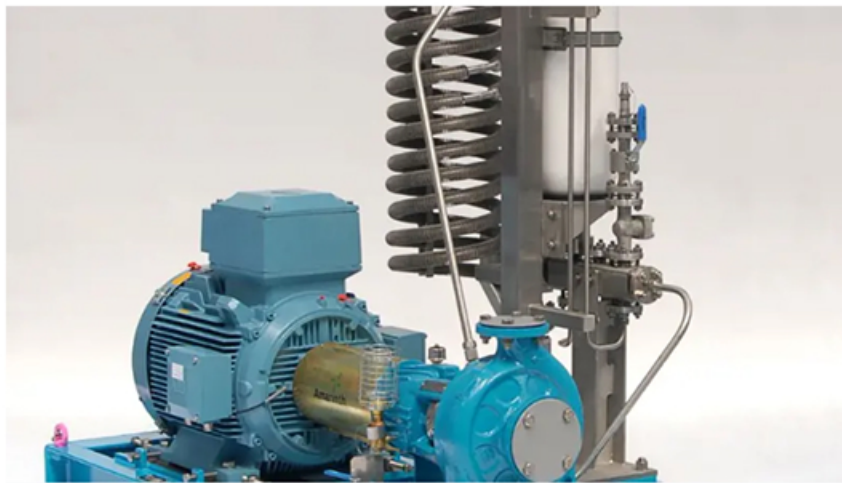
An Amarith API 610 OH1 pump with API 682 Plan 53B seal support system.
