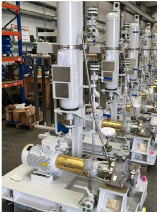
Amarinth API 610 OH2 pumps being assembled for Karachaganak Petroleum Operating. (Image source: Amarith Limited)
