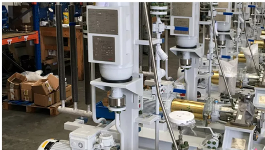
Amarinth API 610 OH2 pumps being assembled for Karachaganak Petroleum Operating (KPO).
