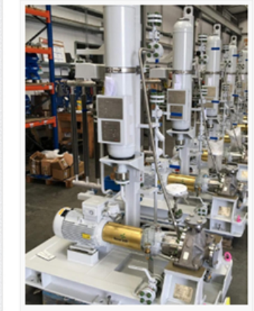
*Amarinth API 610 OH2 pumps being assembled for Karachaganak Petroleum Operating
