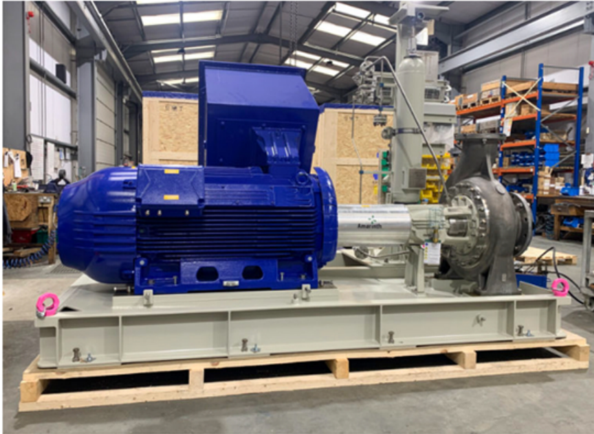
One of the Amarith API 610 OH1 pumps with specialist Plan 53B seal support system being readied for shipment to Cannon Artes. (Image source: Amarith Ltd.)
