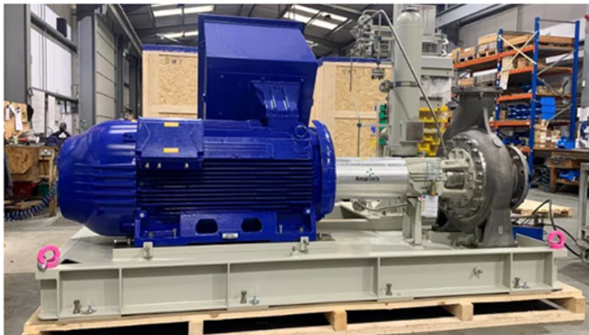
One of the Amarith API 610 OH1 pumps with specialist Plan 53B seal support system prior to shipment to Cannon Artes.
