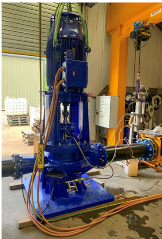
An Amarith API 610 OH3 vertical in-line pump for SICIM undergoing final tests.
