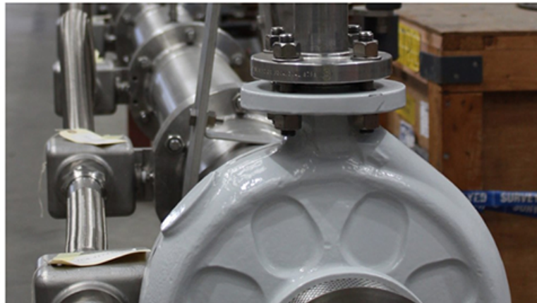
One of the Amarith 18m long API 610 VS4 pumps for the Armada Madura FPSO in assembly – Image: Amarith.
