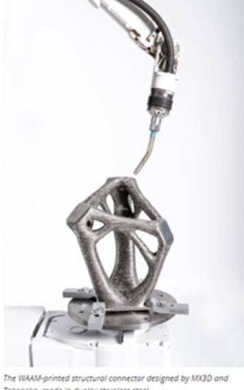
The WAAM-printed structural connector designed by MX3D and Tokenoa, made in duplex stainless steel.
