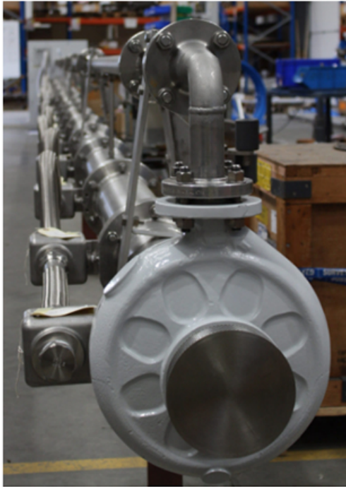
One of the Amarith 18m long API 610 VS4 pumps for the Armada Madura FPSO in assembly (Image source: Amarith Limited)
