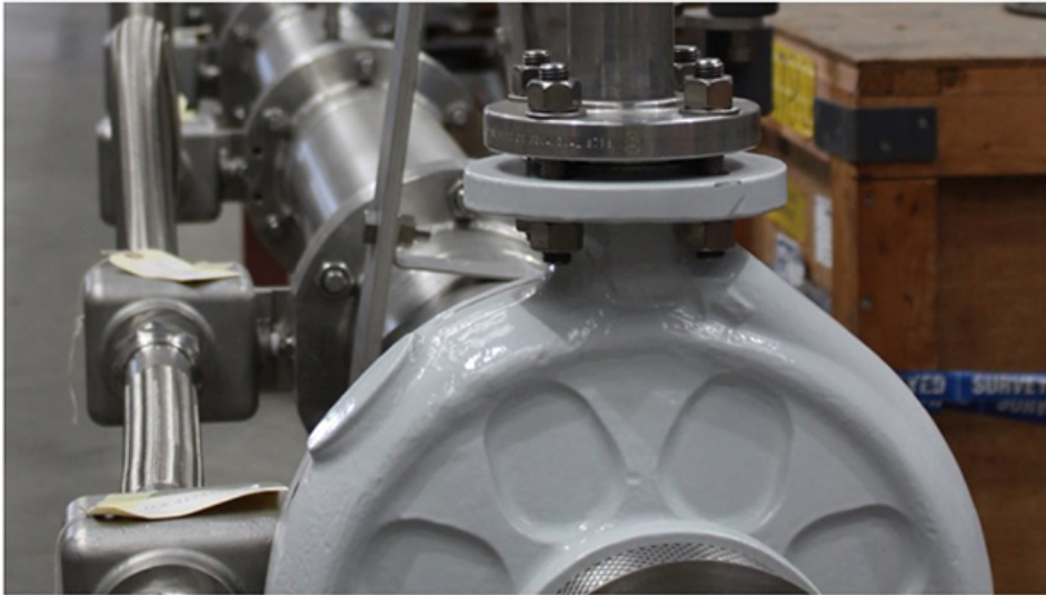
One of the Amarithh 18m long API 610 VS4 pumps for the Armada Madura FPSO in assembly - Image: Amarithh.
