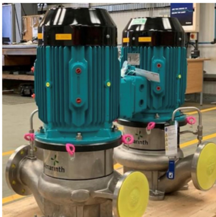
Amarinth vertical in-line pumps ready for shipment to EDF Sizewell B nuclear power station. (Image source: Amarith Ltd.)
