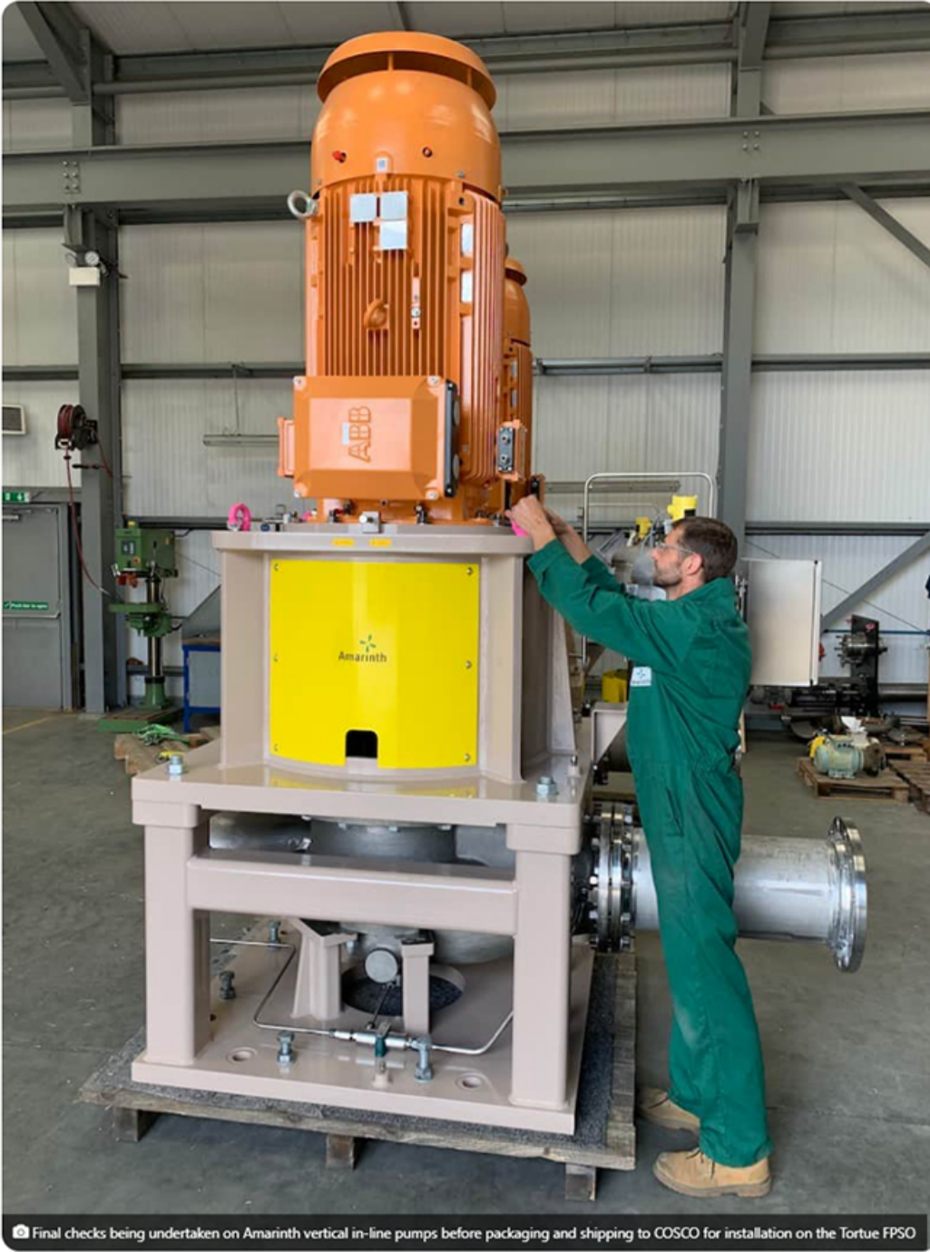
Final checks being undertaken on Amarith vertical in-line pumps before packaging and shipping to COSCO for installation on the Tortue FPSO
