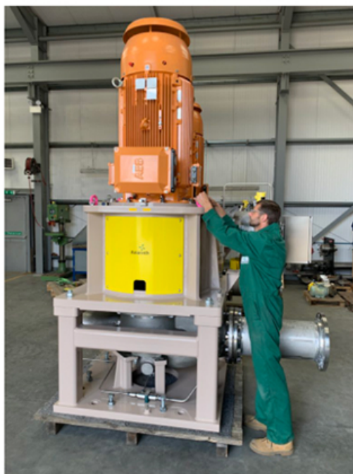
Final checks being undertaken on Amarith vertical in-line pumps before packaging and shipping to COSCO for installation on the Tortue FPSO. (Image source: Amarith Ltd.)
