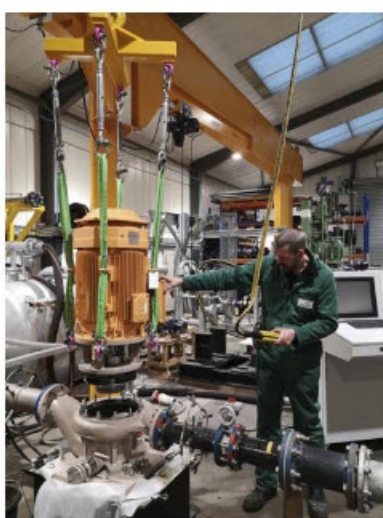
Figure 4. Lowering the motor onto an Amarith vertical inline pump.
