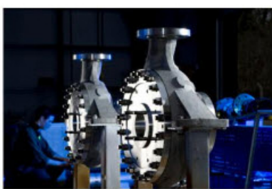
Figure 2. Bespoke strengthened pump castings from Amarith.
