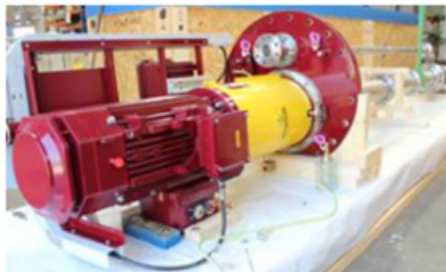
An Amarith API 610 VS4 pump being readied for delivery to the ADNOC Bu Haseer full field development project.
