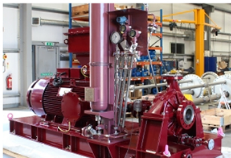
The API 610 OH2 horizontal pumps consisted of a scrubber condensate pump and a production separator pump. (Image source: Amarith)
