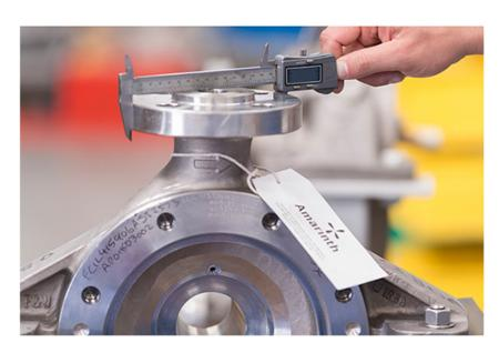
During the Covid-19 pandemic, Sellafield turned to us for a dimensionally and hydraulically interchangeable pump to replace their existing Girdlestone self-priming pump. We were able to provide a bespoke version by taking one of our dimensionally interchangeable pumps and redesigning the casing and impeller to ensure an exact match to the existing pump's hydraulic performance.
