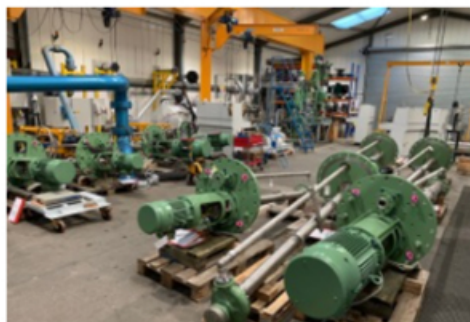
Amarinth API 610 VS4 vertical pumps undergoing testing before shipment. (Image source: Amarith)
