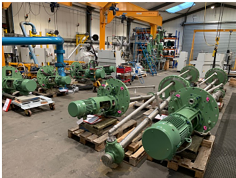
Amarinth API 610 VS4 vertical pumps undergoing testing before shipment (Image source: Amarinth Ltd.)
