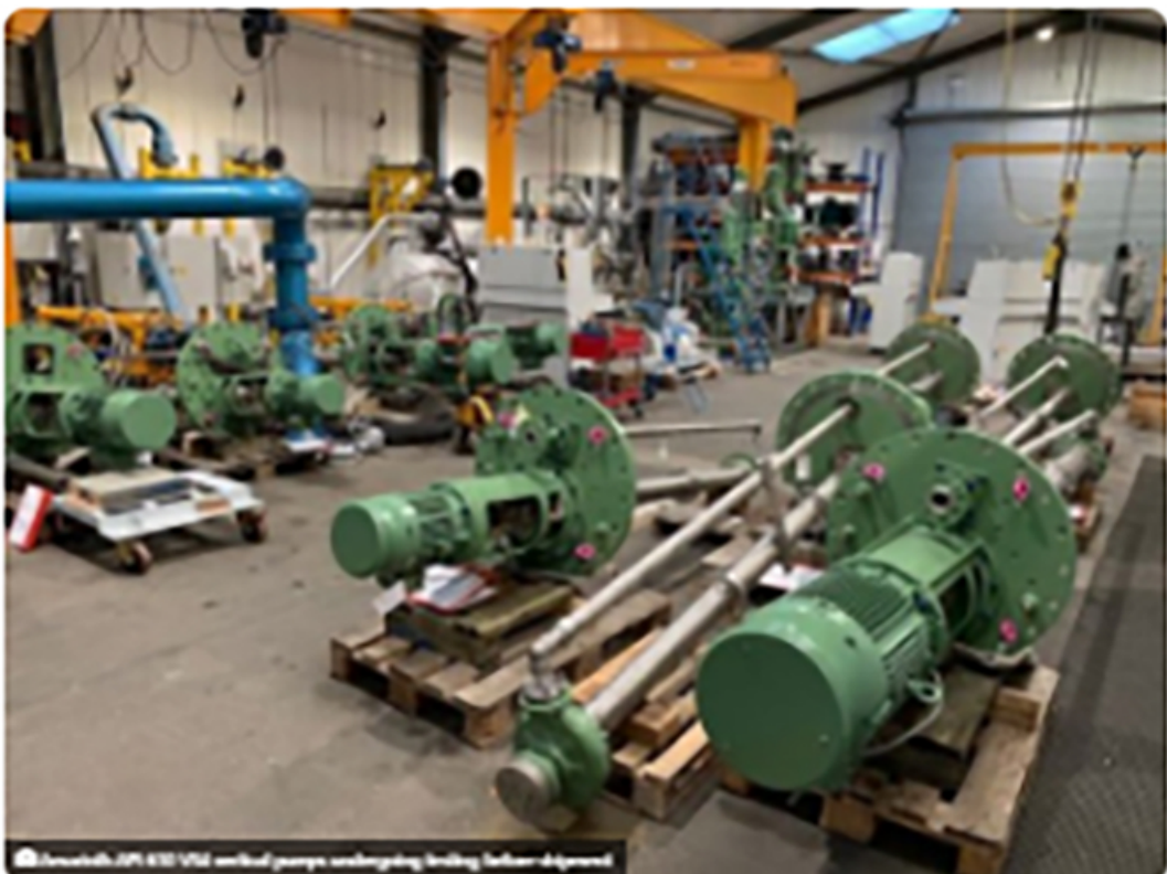
Amarinth API 610 VS4 vertical pumps undergoing final inspection
