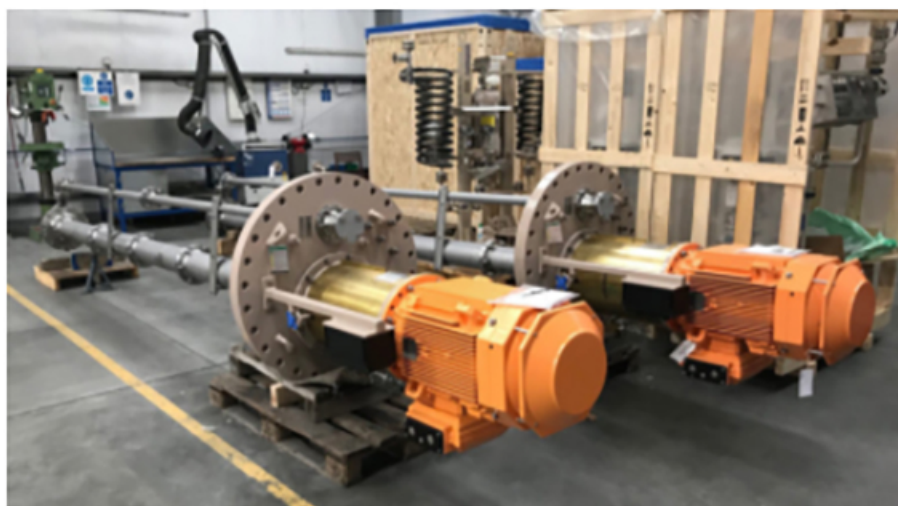
Amarinth API 610 VS4 vertical pumps with Plan 53B seal support systems being readied for shipment to the Garraf Oil Field Development, Iraq (Image source: Amarith Limited)
