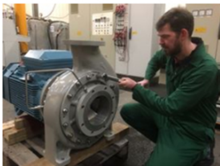
Final assembly of an Amarith nutshell filter pump.
