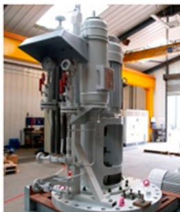
Amarinth API 610 VS4 Pump in assembly. (Image source: Amarith)
