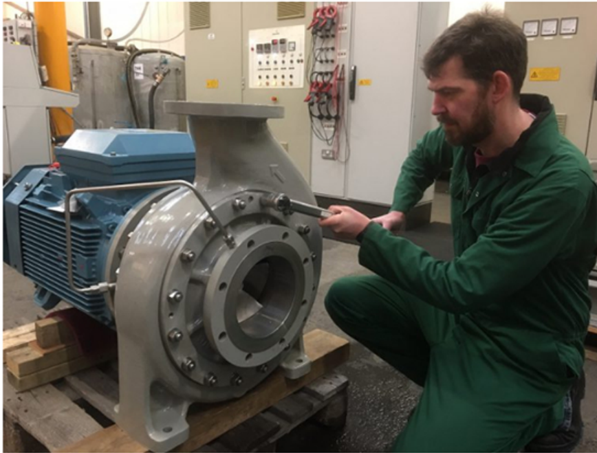
Final assembly of an Amarith nutshell filter pump. (Image source: Amarith Ltd.)
