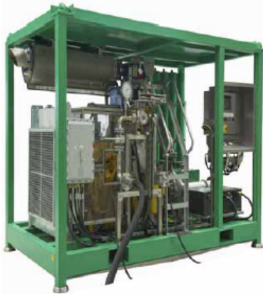
Figure 1. Compact skid packaging of a bespoke gas driven pump.
